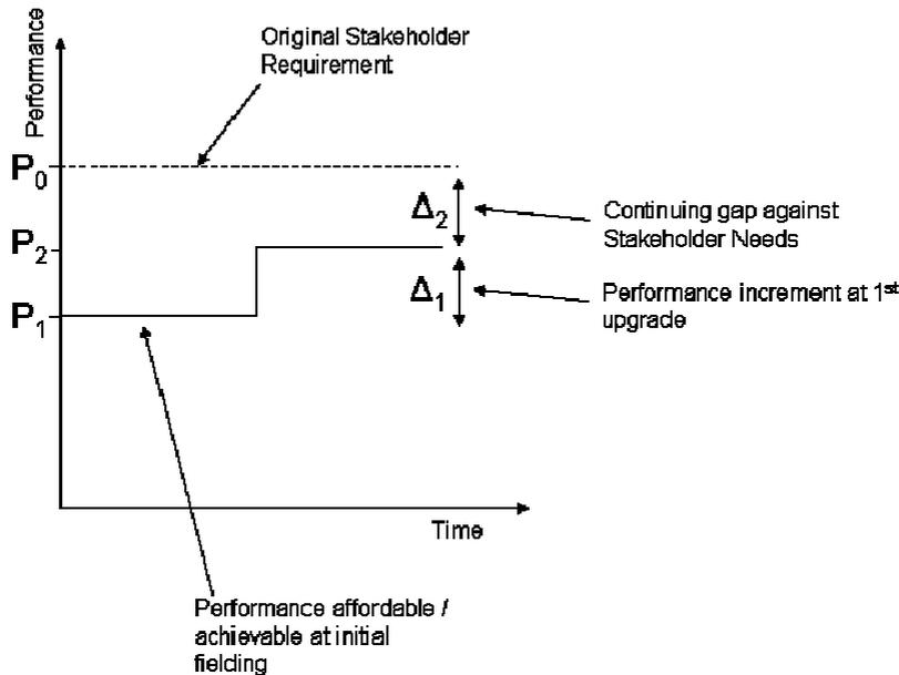
**Figure 5-2: Required system performance may be unachievable initially**
