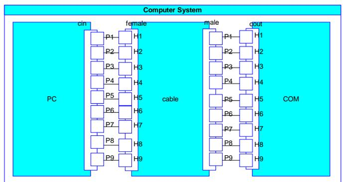
is made up of a Personal Computer (PC), and a COM device, which is an instance of a Modem, which is connected together by the cable. Flows can also be shown on the links, if required. As with the rest of SysML, work is still being done on these diagrams and may change before the final specification is released. This is currently scheduled for August 2004.
